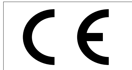
The CE mark, which may not be less than 5mm in height.
