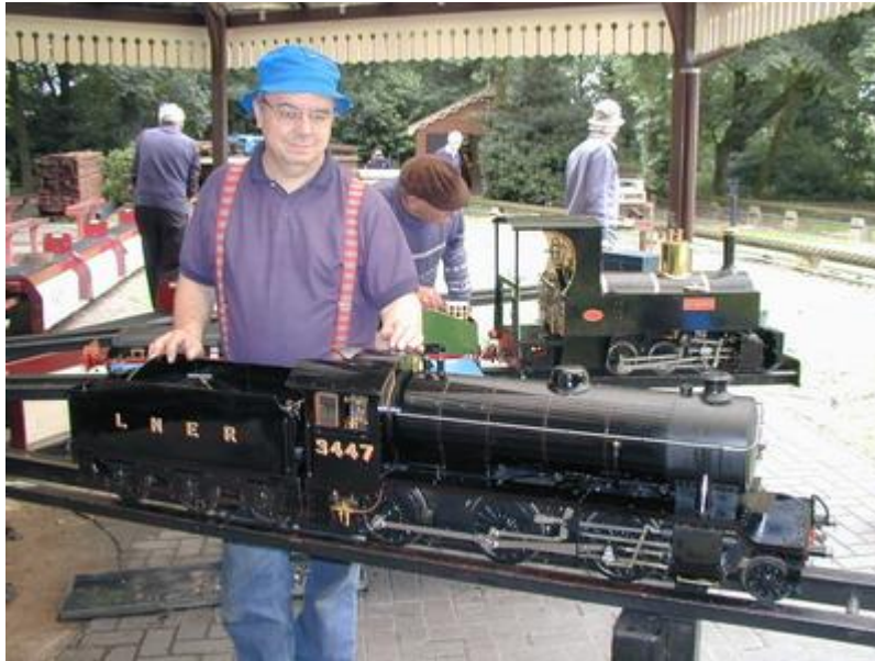
3. A doubled up LBSC Dyak was the basis for Roger James' Freelance 2-6-0, but with a Thompson-type boiler and cab. Roger travelled up from NW Leicester (Coalville) for the occasion.
