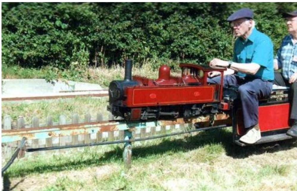
Dave Roberts drives his 5" gauge Beyer Peacock 0-6-2 loco of the La Guarera Y Caracas Railway of Venezuela.
