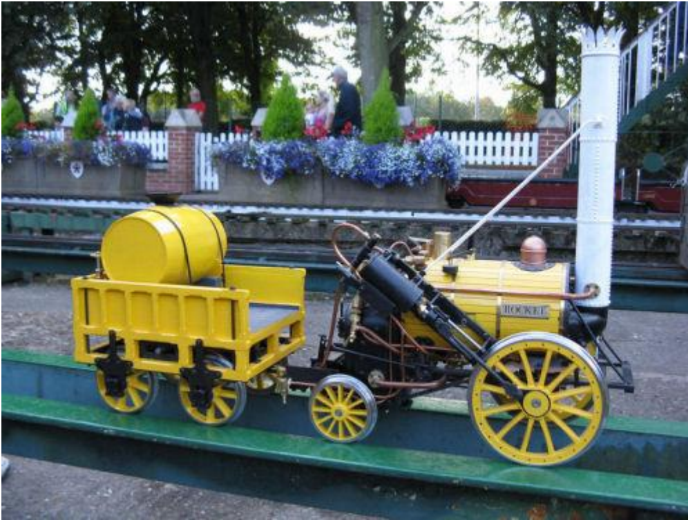
This very nice model of Rocket was built from an OS kit by Ray Wallis, Hon President of LSME. All the metal parts were machined, but Ray still had to do the woodwork, painting and assembly . A very attractive model. The OS kits are very well made and good value, but why do they have to use a massive model style safety valve, instead of suitably adapting the prototypical valve?
